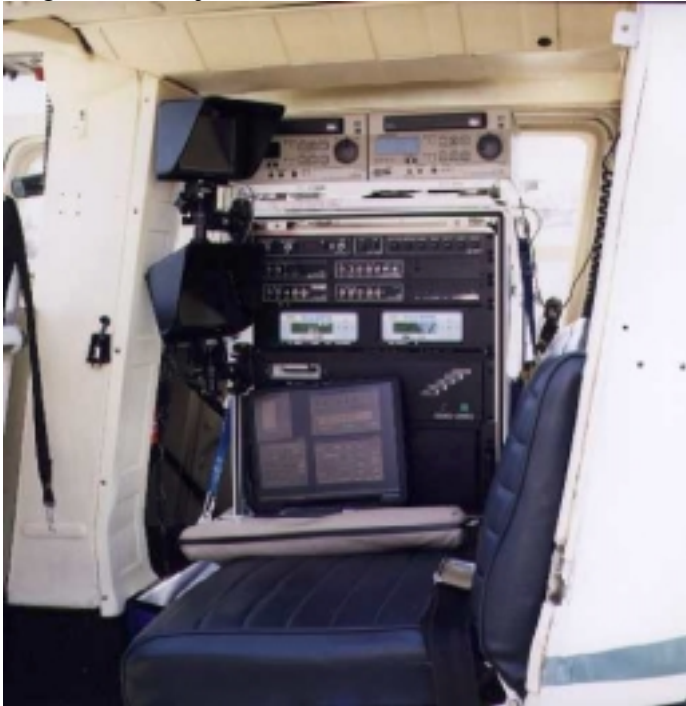
FLI-MAP ® equipment inside helicopter
