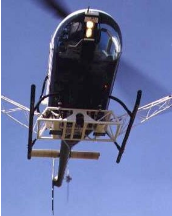
The FLI-MAP helicopter with the two eye-safe lasers
