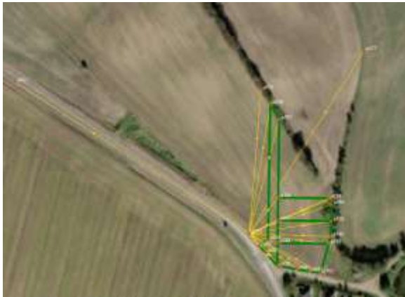
Figure 14a. Set-out of new boundary points from control point -022
