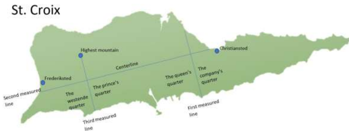
Figure 2 The figure shows the first lines that were surveyed on St. Croix. The lines are shown in blue and Christiansted, the highest mountain, and the neighborhoods are indicated in the figure. The figure is for illustration only and therefore not measurable.
