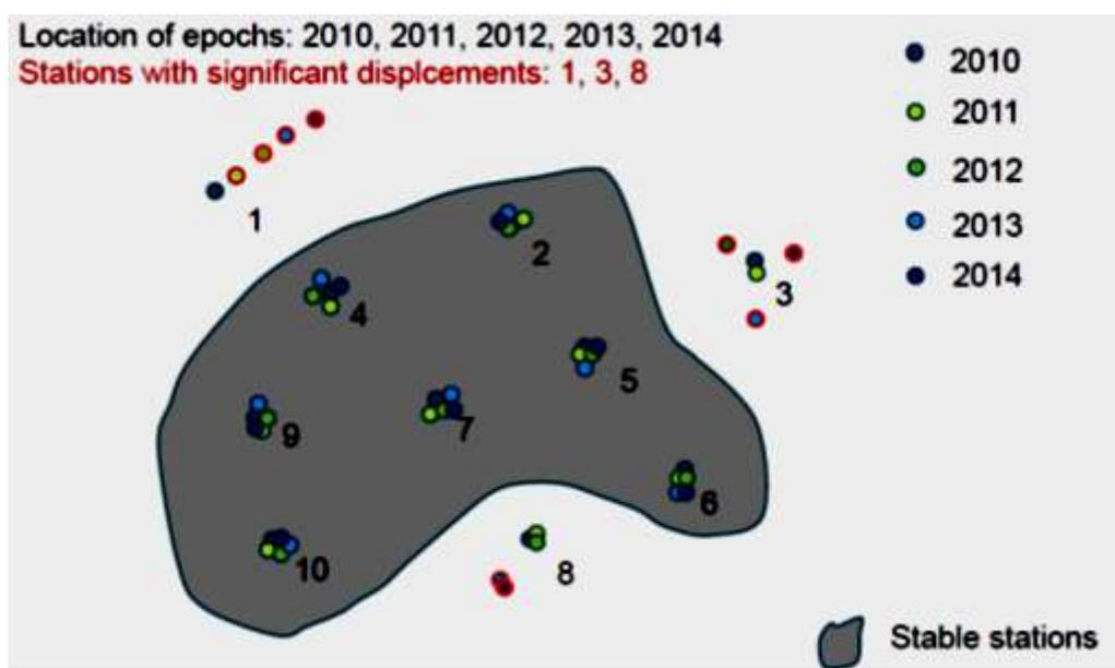
Fig. 3: Extension of the classical congruency tests to derive movement pattern out of the analysis of several epochs (Tengen et al., 2019)
