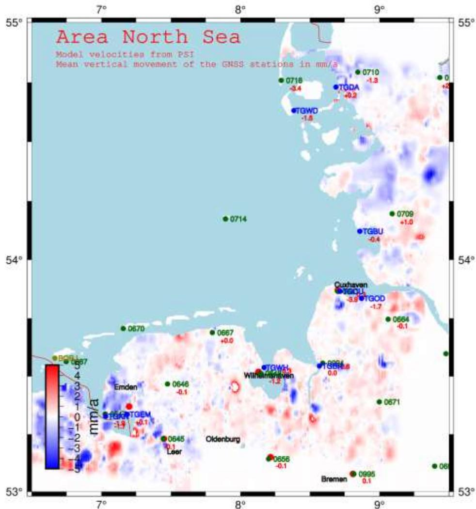
Fig. 8: Vertical movements for Northern Sea in Germany, derived out of PSI data 2014-2019
