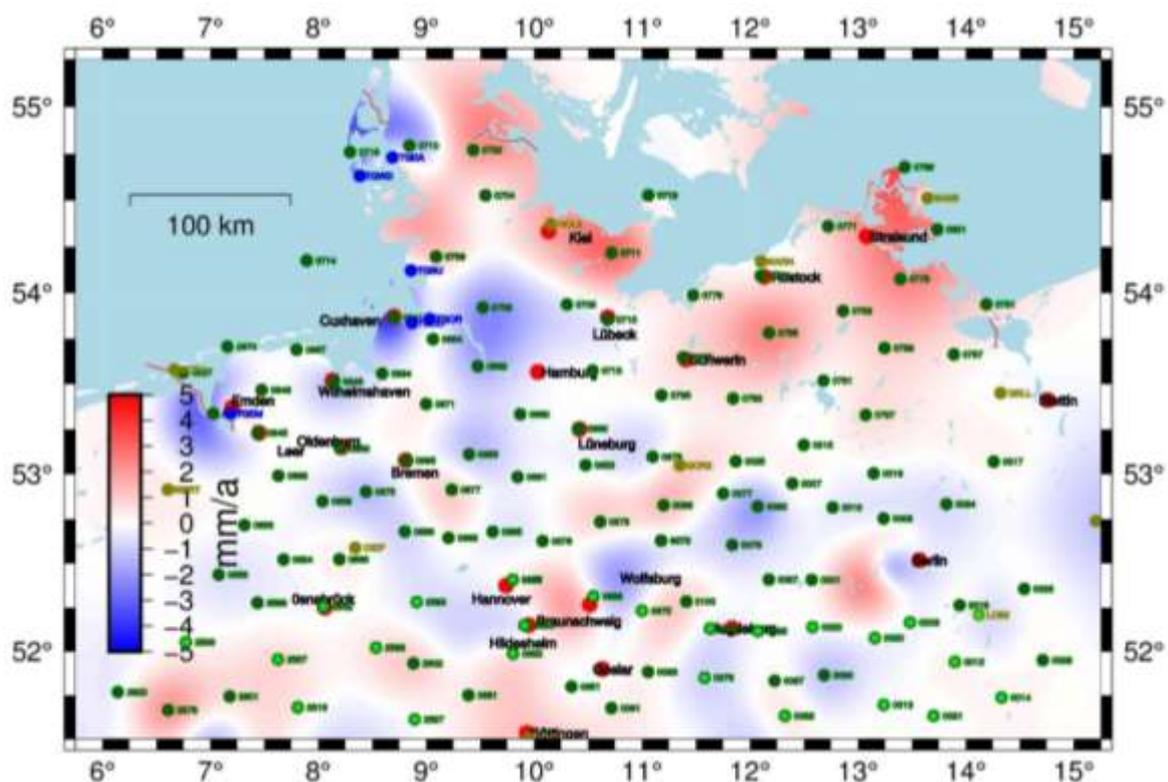
Fig. 7: Velocity field for vertical movements, derived out of GNSS time series 2010 - 2016
