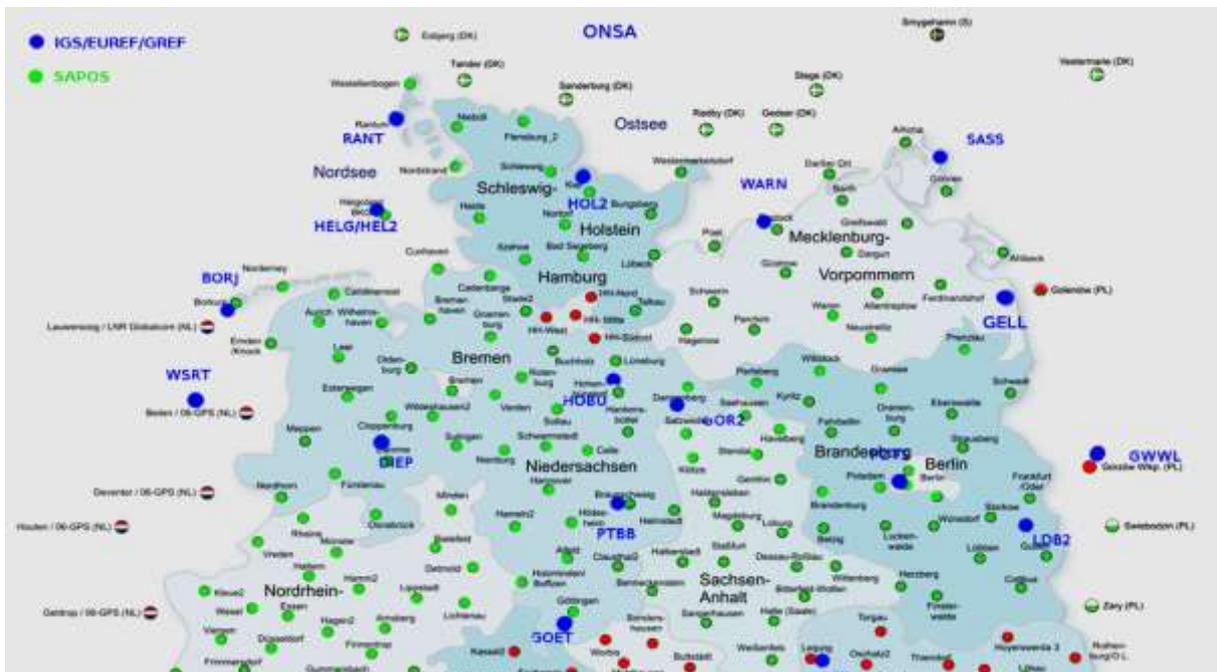
Figure 1: Location of GNSS permanent stations included in this project. Aside of SAPOS stations the reference group with IGS, EUREF and GREF stations are depicted.
