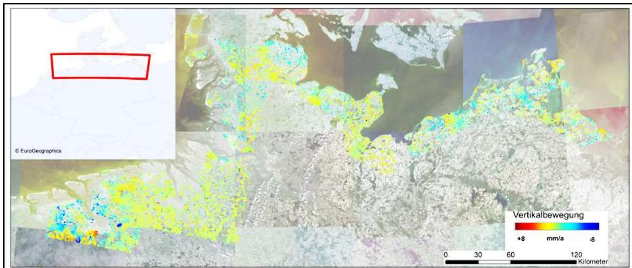
Fig. 5: Combined result of the PSI-analysis for the coastal areas of Northern and Baltic Sea in Germany, derived as linear model for the time span Oct. 2014 to Febr. 2019.
