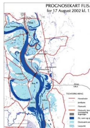
Dynamic Flood inundation warning map
