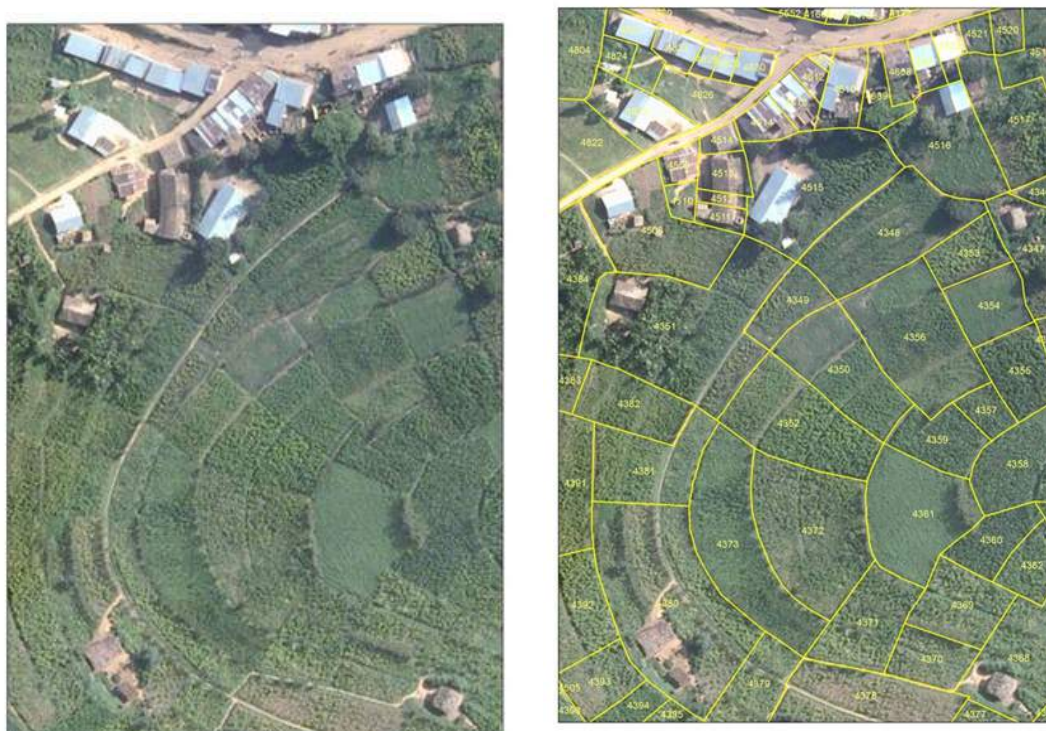
Figure 6: Example from Rwanda showing and aerial imagery (left) from which the parcel boundaries are easily identified (right). Source: Didier Sagashya, Rwanda
