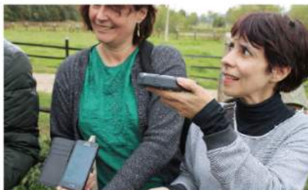
▲ Figure 2, The Trimble R1 has a Bluetooth connection with a mobile on which also Esri's Collector App is installed.
