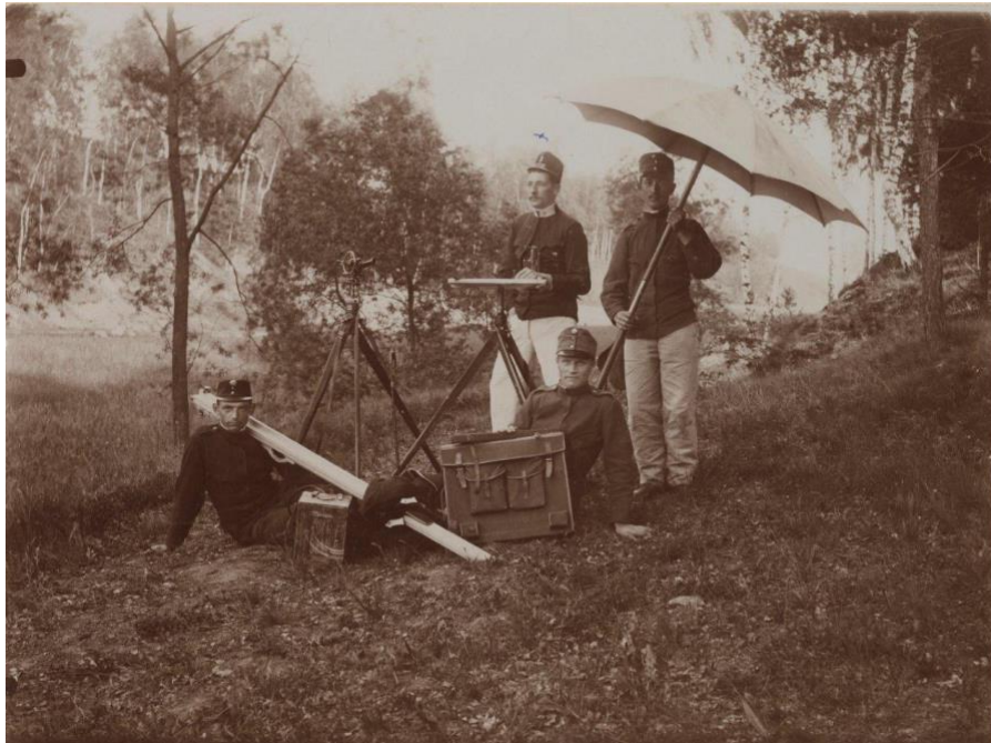
Figure 7: Surveying team in France, 1908, using theodolites for fixing a control point and plane tables for recording topography and parcel boundaries.
