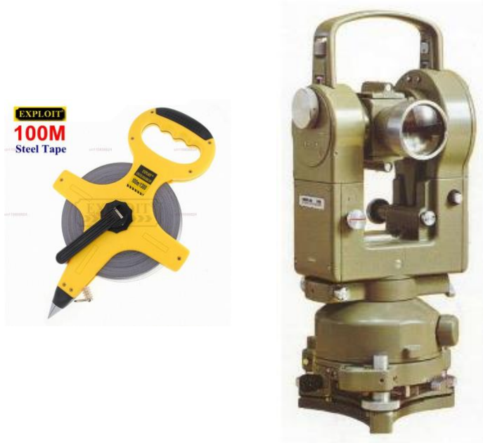
Figure 10: Wild T2 Universal Theodolite (Pictures from the Archive of the Wild Heerbrugg AG, apart from the tape which was found from general Internet search)
