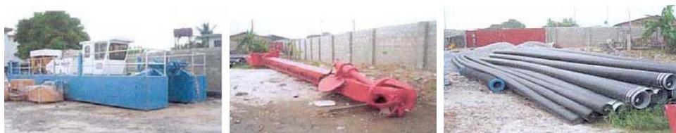
**Figure 4b:** A 12" x 10" ellicott truckable cutterhead suction dredge powered by a 370 hp caterpillar diesel engine, with a 10m ladder and maximum digging depth of 6.1m. Included are 500 metres of 12 inch hdpe pipe with 300 metres of 8 inch hdpe floats.
