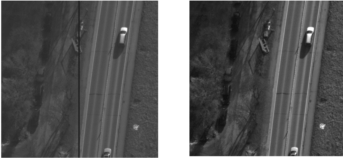
Figure 6: Image cut containing a defect column (left) and corrected image (right)
