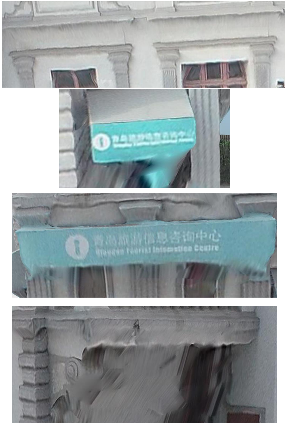
Figure 8 UAV aerial image reconstruction model problem
