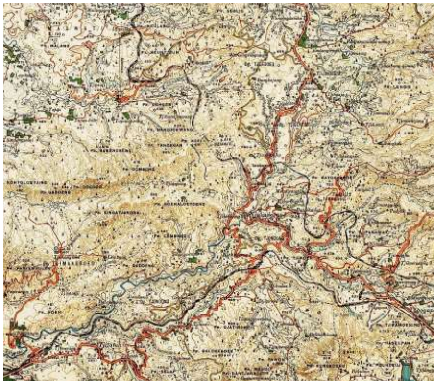
Railways near Padalarang (West of Bandung): junction of the Batavia–Purwakarta–Plered–Padalarang–Bandung railway and the Batavia–Bogor–Sukabumi–Cianjur–Padalarang–Bandung railway, scale 1:50.000 map of 1923.
