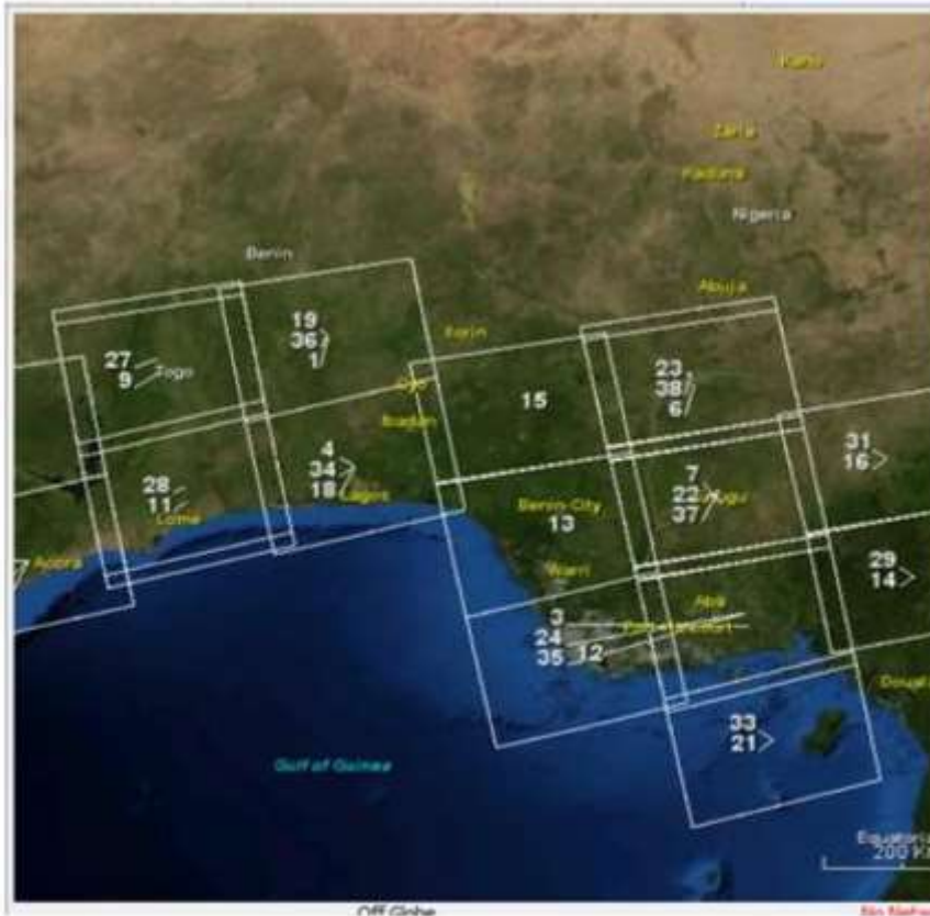
Figure 3: Sample of Interferometric Wide (IW) swath of the study area
