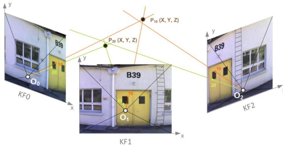
**Figure 3** Schematic illustration of the photogrammetric forward intersection to measure object points  $P_{10}$  and  $P_{20}$ .
