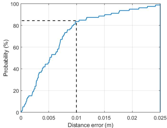
**Figure 8** Error distribution of the distance measurements between two points in the same image group.
