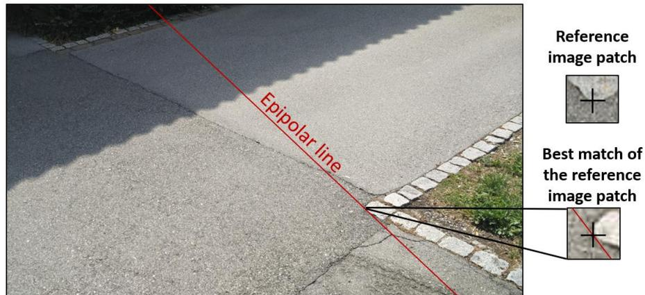
**Figure 4** The matching algorithm searches for the best match of the reference image patch along the epipolar line to find the corresponding points.
