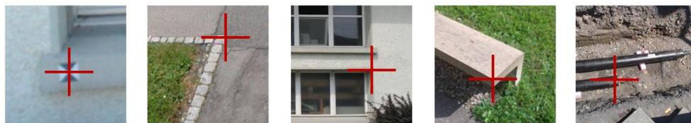
**Figure 5** Examples of the measured object points such as photogrammetric markers, stone edges, window corners, concrete edges and pipes.
