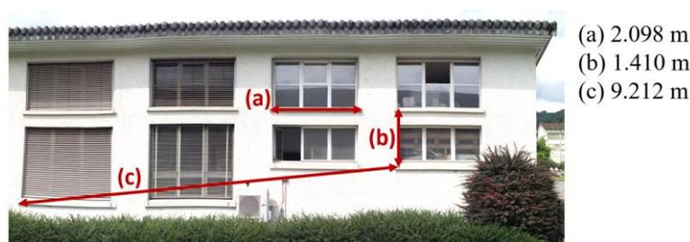
**Figure 7** Defined reference distances on a building facade for evaluating the relative accuracy of the image-based surveying system.
