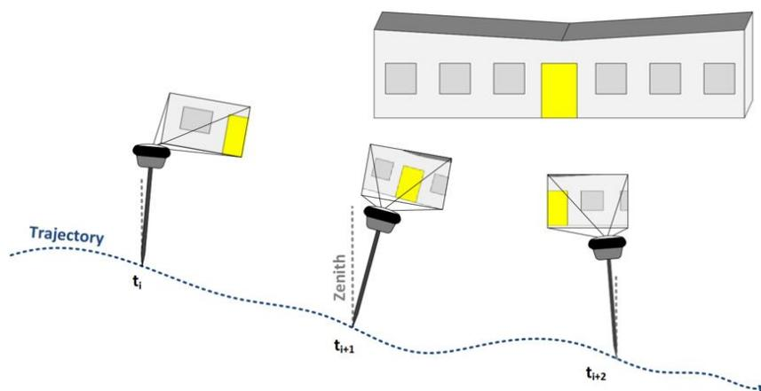
**Figure 1** Schematic illustration of the measurement workflow of the presented image-based surveying approach, where images are recorded at epochs ( $t_i, t_{i+1}, t_{i+2}, \dots$ ) while passing the scene of interest.
