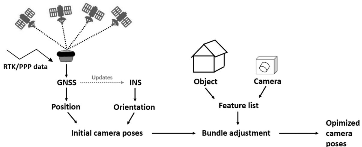
**Figure 2** Flow diagram representing the optimization process of the camera pose estimation.
