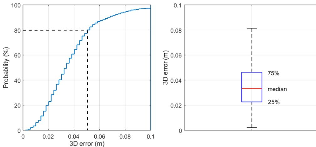
**Figure 6** 3D error distribution of 1075 image-based remote point measurements shown in empirical cumulative distribution function (CDF) and boxplot.
