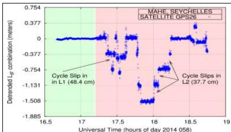
**Figure 5. Cycle-slips on actual GNSS carrier-phase measurements caused by ionospheric scintillation.**
