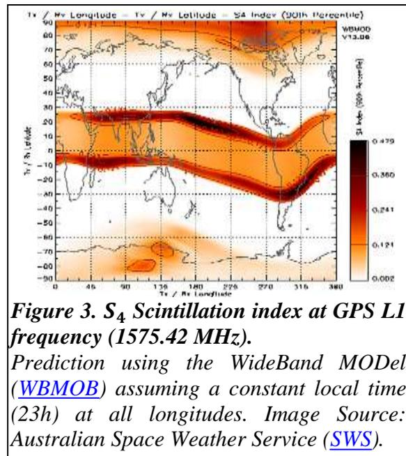
**Figure 3.  $S_4$  Scintillation index at GPS L1 frequency (1575.42 MHz).**
