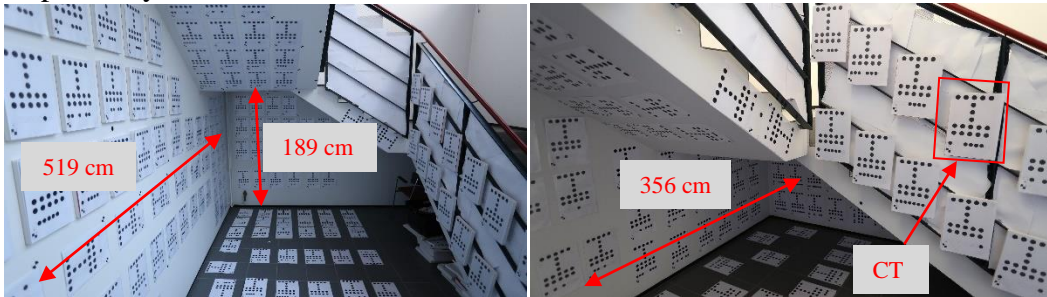
Fig. (4) Side view of the calibration room at FGI. Coded targets (CT) are installed on all surfaces.
