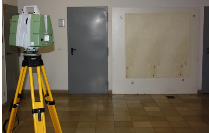
Fig. 3: Measurement configuration when scanning the wooden panel
