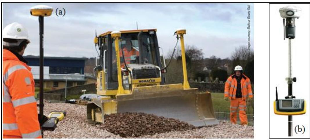
**Figure 2:** (a) GNSS-Activated leveling bulldozers: (b) Trimble Integrated surveying combines robotic total station with RTK GNSS ([www.trimble.com](http://www.trimble.com))
