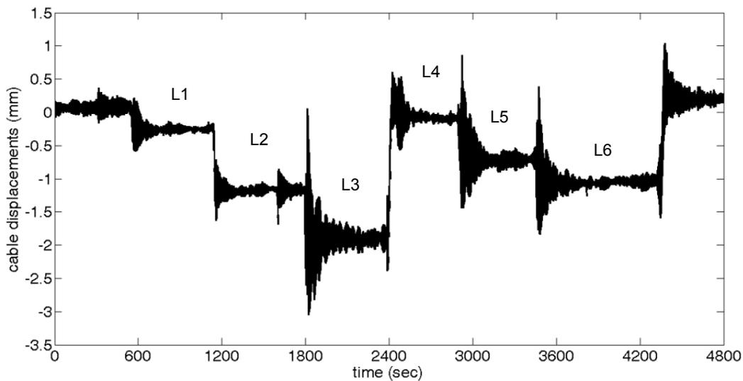
**Figure 7.** Displacements of the third (longer) cable perpendicular to the cable axis at distance approximately at one third of cable length measured from the top of the pylon
