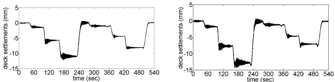
**Figure 5.** Deck settlements at third (longer) cable anchor point area obtained by DIC and GBMI systems for all load test positions
