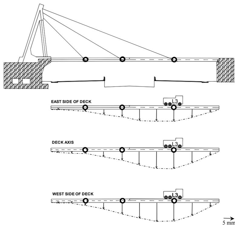
**Figure 4.** Deck settlements derived from precise leveling for test load L3, see Fig. 2
