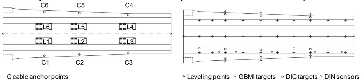
**Figure 2.** Loading scenarios (left) and sensor placement (right)
