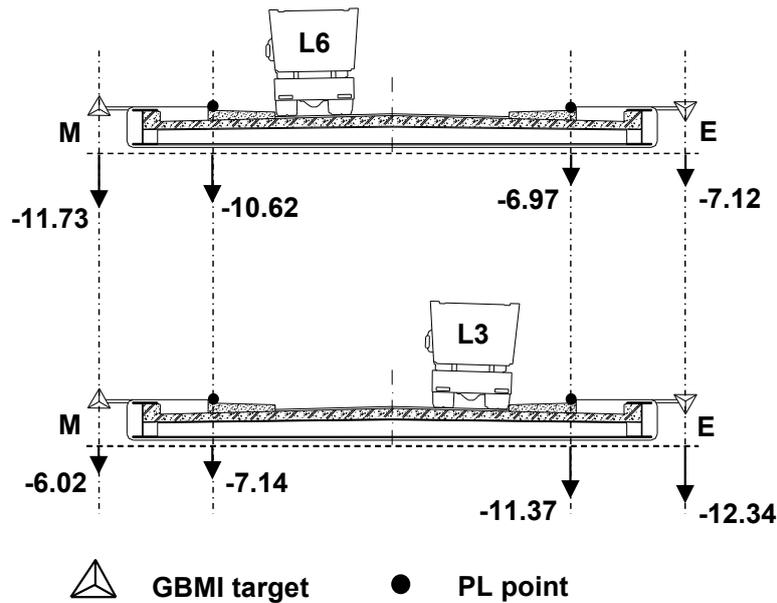
**Figure 6.** Deck settlements in millimeters obtained at the GBMI and DIC targets located in the proximity of track position for load cases L6 (top) and L3 (bottom)
