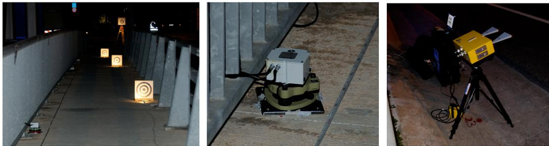
**Figure 3.** DIC targets, digital inclinometer (left) detail of digital inclinometer (center) and GBMI sensor (right)
