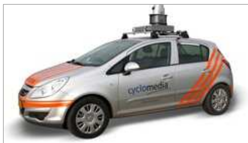
Figure 3. Surveying car with photographic equipment (Cyclomedia 2012)
