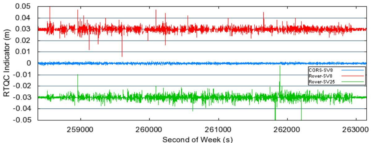
Figure 7. Individual RTQC Indicators during railway survey on 4<sup>th</sup> March 2009.
