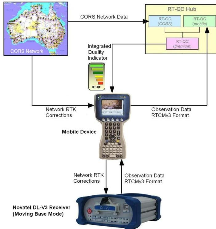
Figure 4. Novatel Moving Base Set Up.
