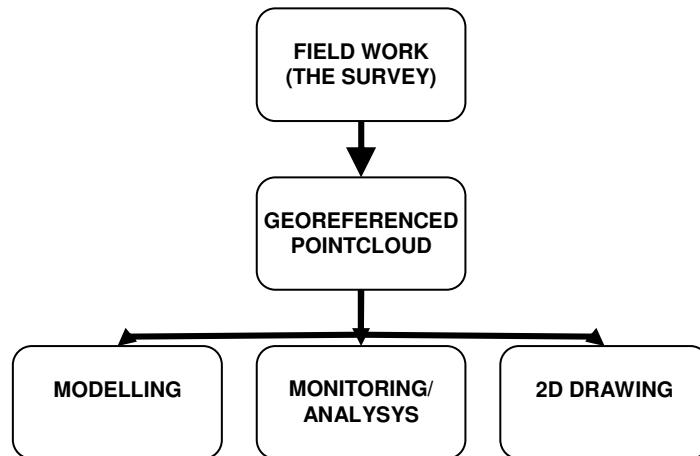
**Schematic view 1.1** 3D scanning processing steps
