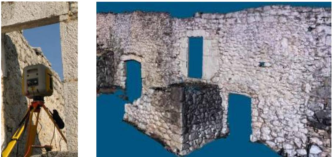
**Figure 1.2** Trimble GX 200 during measuring in Dobranje (left) and a part of the measured point cloud (right)
