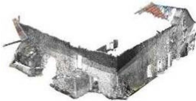
**Figure 3.3** Aligned and merged point clouds
