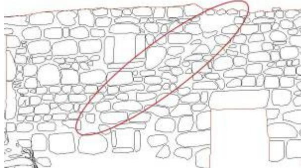
**Figure 3.8** Traces of a former roof
