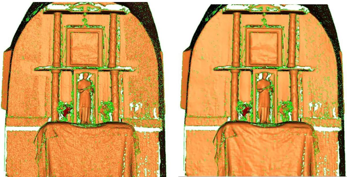
**Figure 3.6** Mesh after creation (left); Mesh after smoothing and noise reduction (right)
