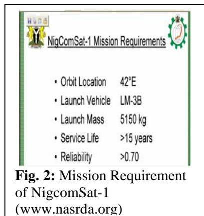
**Fig. 2:** Mission Requirement of NigcomSat-1 (www.nasrda.org)
