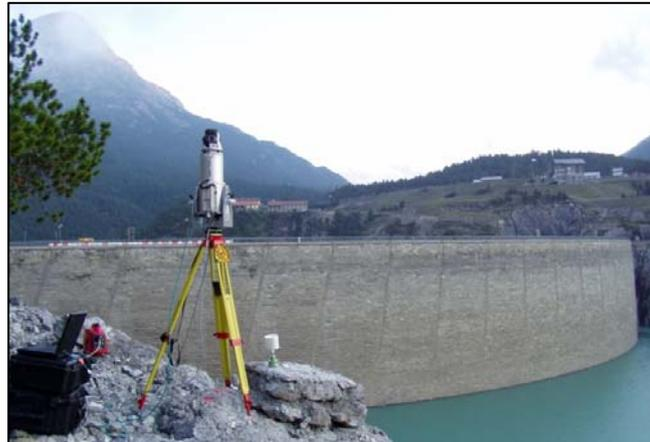
**Figure 4:** laser scanner Riegl LMS-Z420i with its tools during scanning of the dam downstream face.
