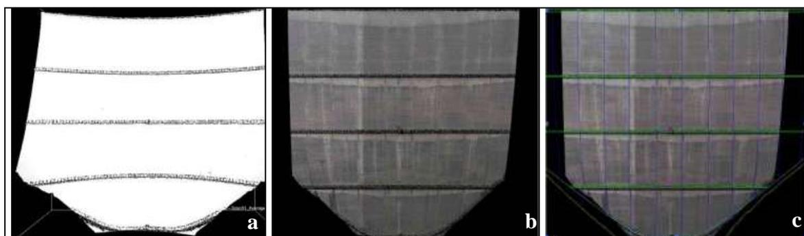
**Figure 4:** process to generate a vector prospect of the central portion of the dam downstream face (from left to right): triangulation (a), ortoprojection (b), vectorization (c).
