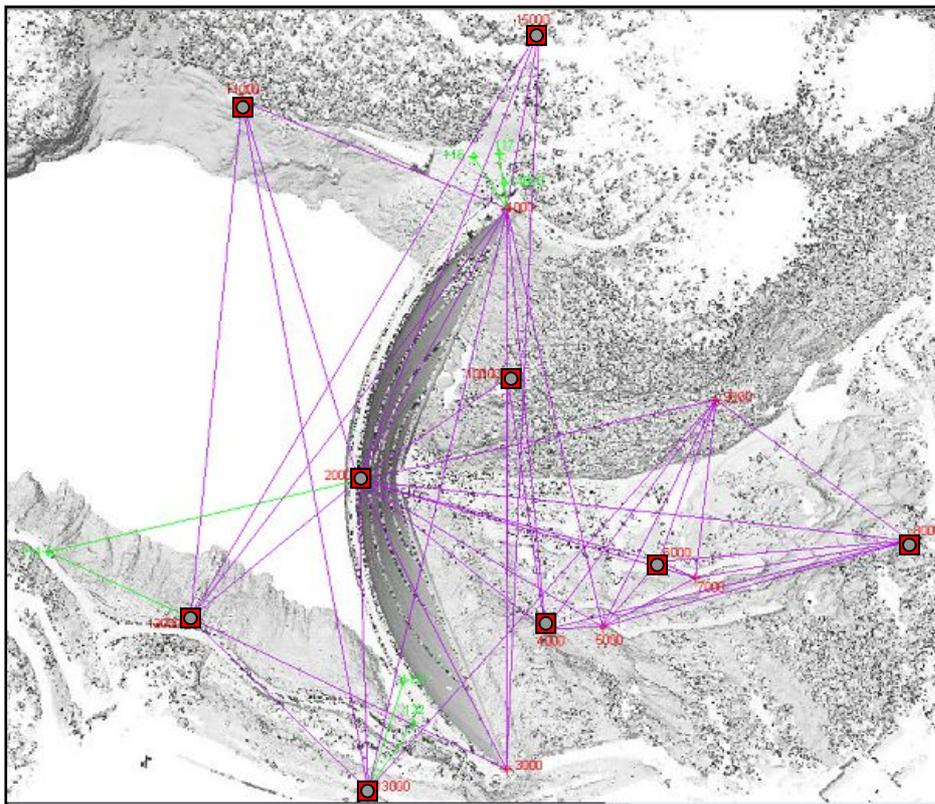
**Figure 2:** planimetric view of the dam of Cancano Lake, reporting the layout of the geodetic network and the main laser scanning stand-points.
