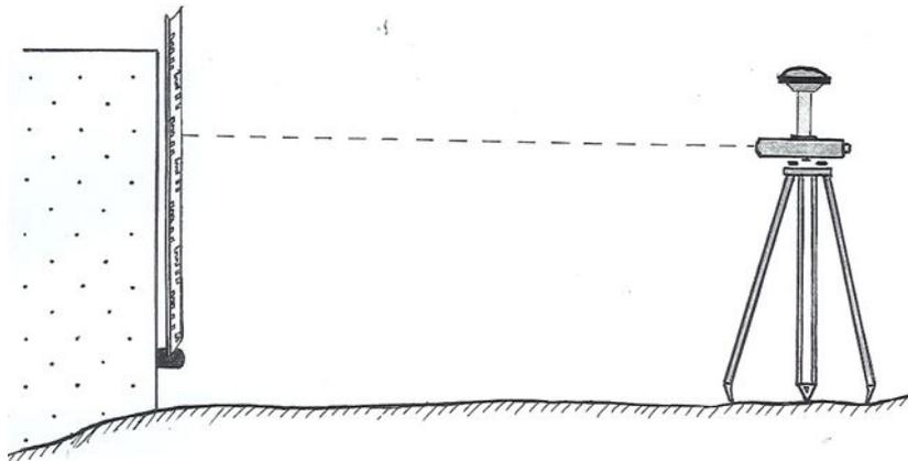
**Figure 2** - GNSS antenna mounted on a level observing staff on a wall-benchmark
