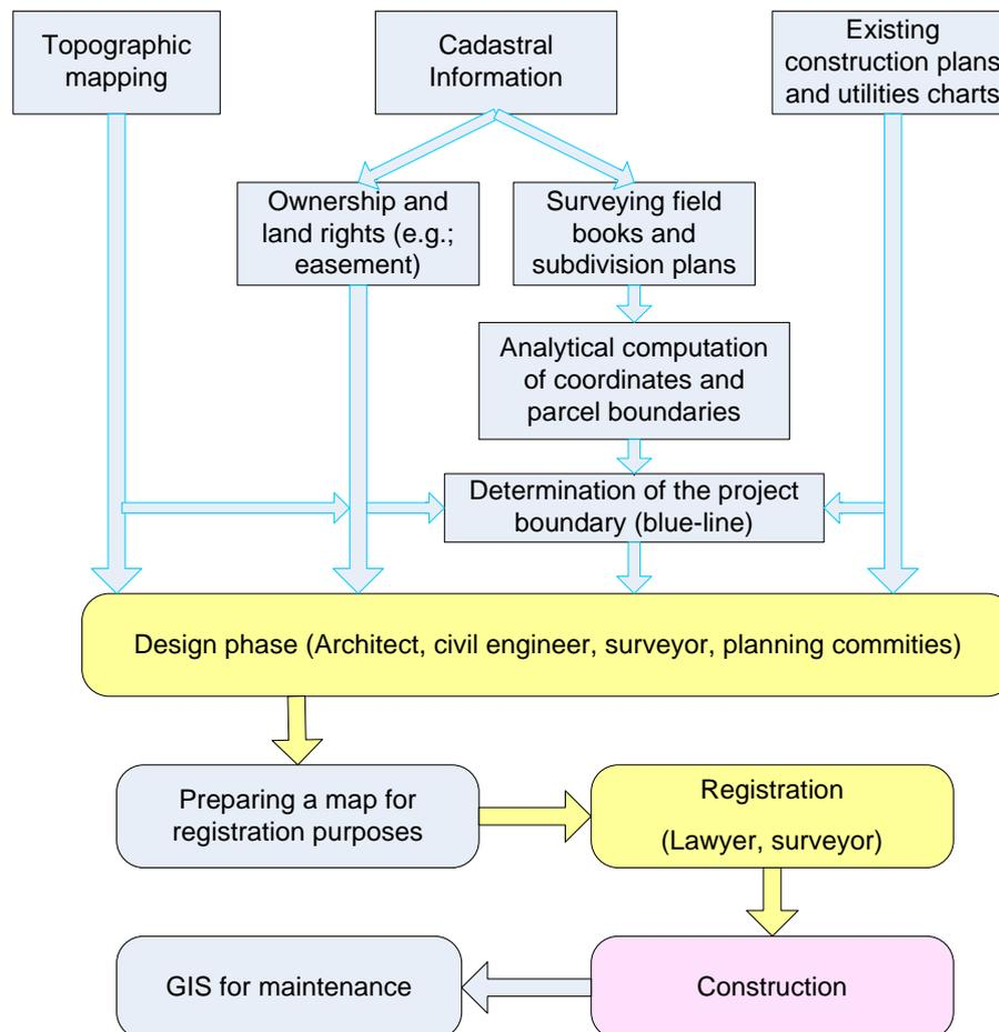
**Figure 1:** The different steps in the urban development workflow. Blocks in light blue are tasks that are performed by the surveyor.
