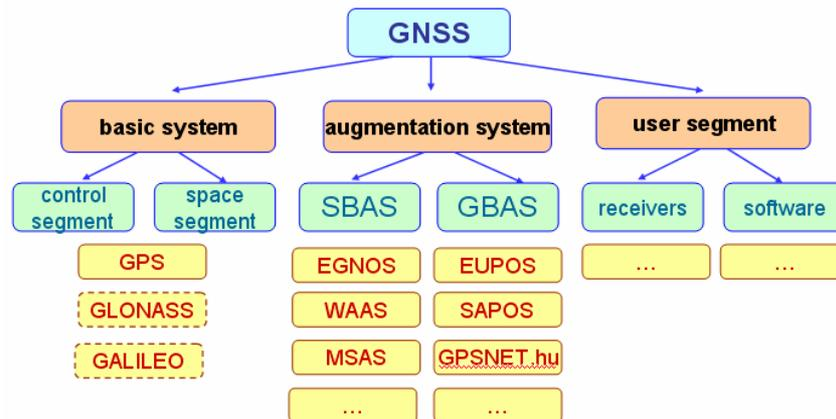
Fig. 1. The components of GNSS
