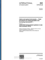
This standard specifies field procedures to be adopted when determining and evaluating the precision (repeatability) of Global Navigation Satellite System (GNSS) field measurement systems (this includes GPS, GLONASS as well as the future systems like GALILEO) in real-time kinematic (GNSS RTK) and their ancillary equipment when used in building, surveying and industrial measurements.
