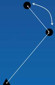
Measure the distances and height differences between the two rover points are measured by independent methods to a precision of better than 3 mm.
