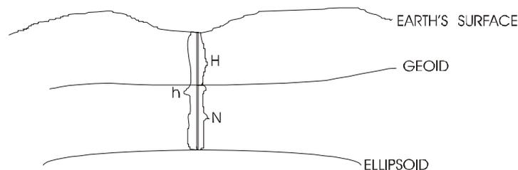
FIG. 2: Relationship between the ellipsoid, the geoid and the earth's surface
