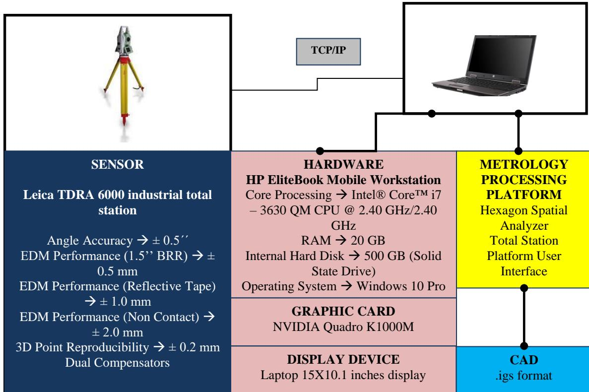
Fig.2: System architecture
