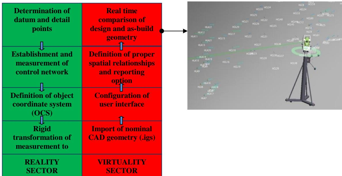
Fig.3 Case study of an AV-LSM workflow
