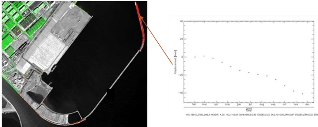
*Fig. 4 Time series over the southern dike with RADARSAT*
