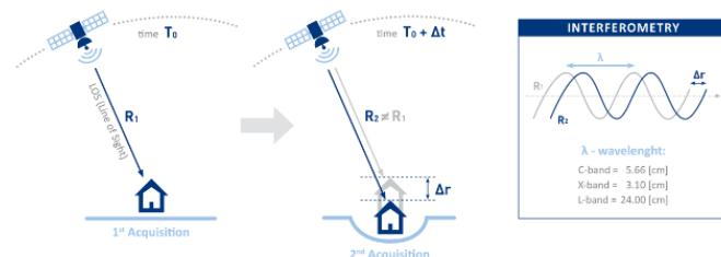
*Fig. 1 Schematic showing the relationship between ground displacement and signal phase shift*
