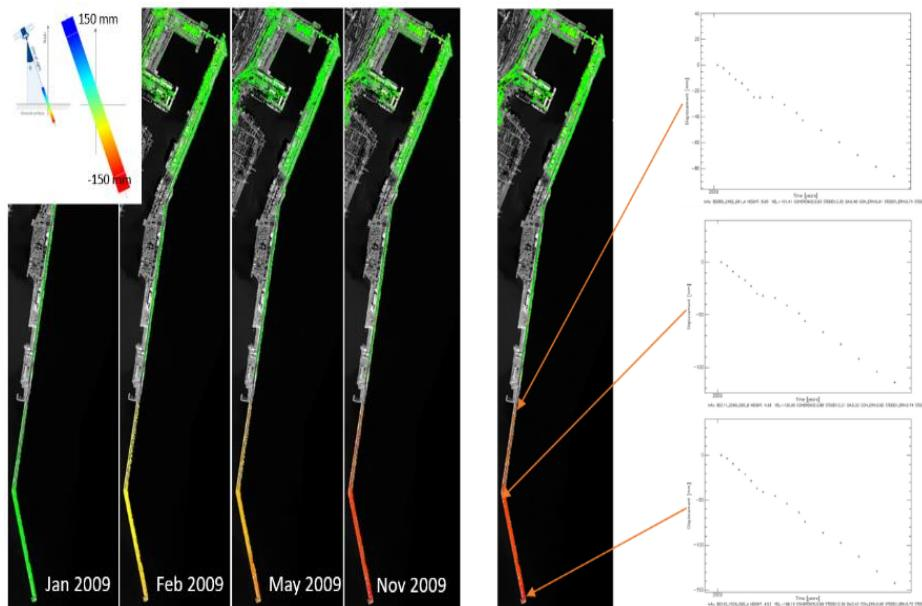
*Fig. 5 Left Temporal evolution of the settlement in LOS (Line of Sight of the satellite) in the eastern dike with TerraSAR-X. Right: TS over the eastern dike with TerraSAR-X.*
