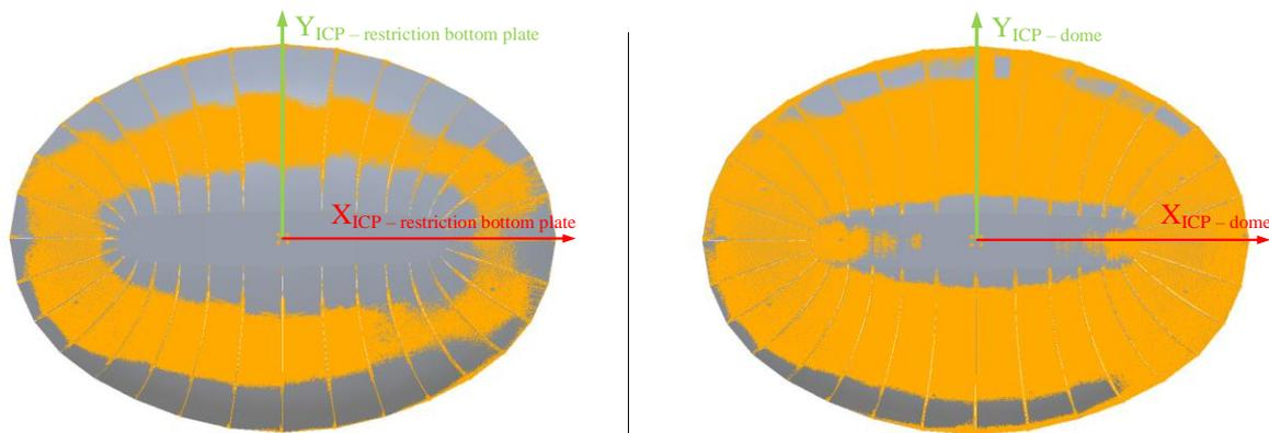
Figure 4: ICP datum differences. ICP – ground plate restriction (left, see 4.1.1); ICP - dome (right, 4.1.2); grey: CAD model; brown: the scanned 3D point cloud
