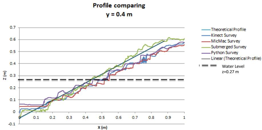
*Fig. 4 Profile comparing using the four methodologies*
