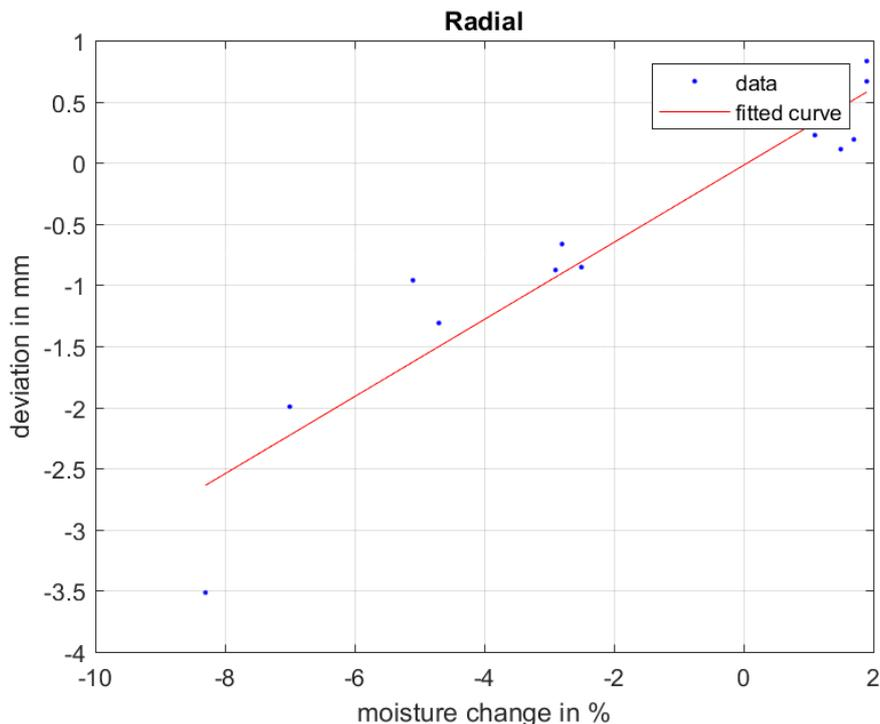
Fig. 4 Deformations due to moisture changes in radial direction
