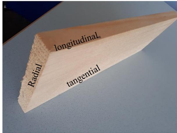
Fig. 3 Example of the used wooden plates
