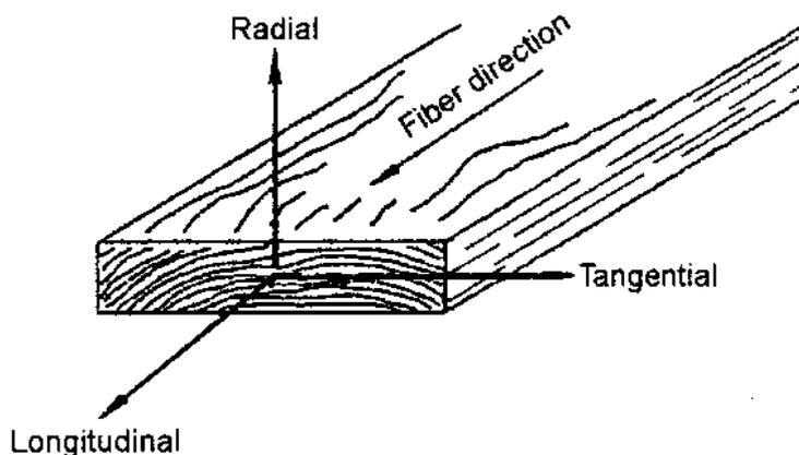
Fig. 2 Axes of wood (Hunt & Gu, 2006)
