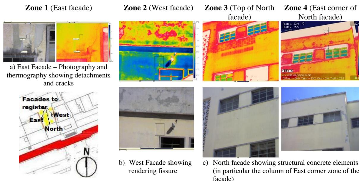
Fig. 8 Use of infrared thermography for the detection and evaluation of anomalies
