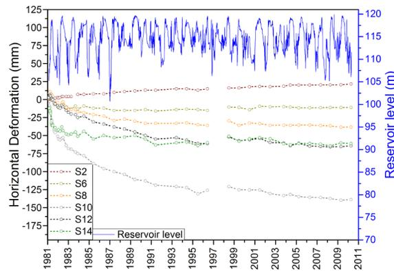
**Fig. 6** Horizontal deformations of the crest control points of Pournari I dam from 1981 until 2010. Positive values indicate deformations towards the downstream direction.
