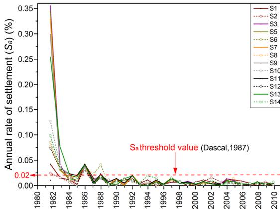
**Fig. 5** The annual rate of settlement of the crest control points from 1981 until 2010 was stabilised below the value of 0.02% in 1989, almost 8 years after the first reservoir filling.
