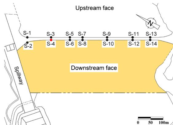
**Fig. 2** Location of control points located on the crest of Pournari I dam (the dataset from S4 was not available).
