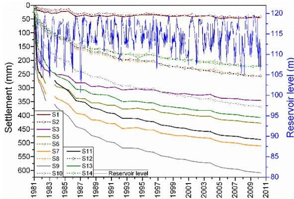
**Fig. 3** Evolution of the settlements of all crest control points of Pournari I dam and reservoir level fluctuations. The upstream side of the crest appears to have the maximum observed settlements. The rate of settlements became more gradual after 1988 when the reservoir drawdown level remained relatively higher compared to the period 1981-1987.
