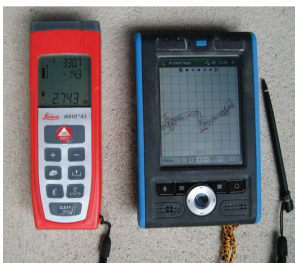
Figure 2 DistoX “paperless caving” system (Paperless Cave Surveying, 2013)
