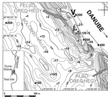
Figure 2 - The contour map of the test site. Circles denote the GPS points (100-600), triangles mark the gravity points (1-21), 10G is the gravity reference point, crossed circles denoted by I and V show the location of the borehole tiltmeters
