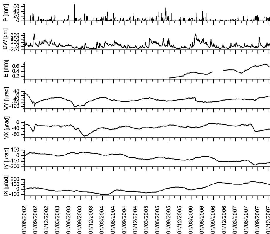
Figure 4 - Data recorded on the Dunaföldvár test site between 06.06.2002 and 31.12.2007. P = precipitation, DW = Water level of the Danube, E = Vertical borehole extensometer, VY = Y tilt component at the foot of the high bank, VX = X tilt component at the foot of the high bank, IY = Y tilt component on the top of the high bank, IX = X tilt component on the top of the high bank
