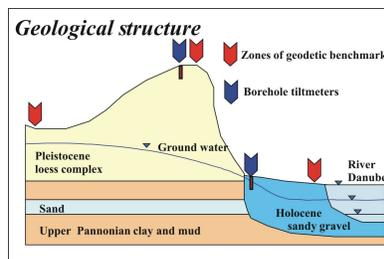
Figure 3 - Simplified geological structure of the test site
