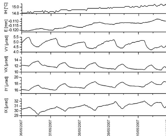
Figure 9 - An example for the short periodic variations in the tilt and extensometric signals. IH = the temperature in the borehole on the top of the high bank; VX, VY = tilt components measured at the foot of the high bank; IX, IY = tilt components measured on the top of the high bank
