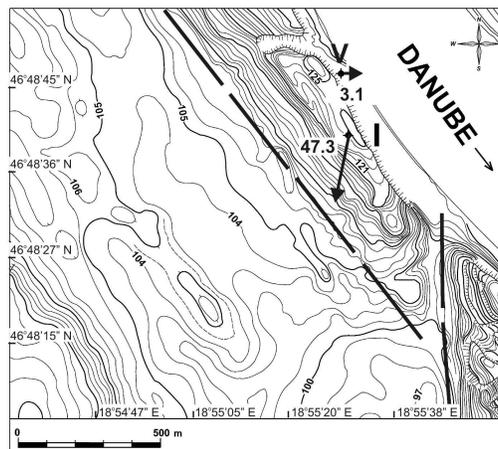
Figure 5 - Tilt rates measured on the top (I) and at the foot (V) of the high bank. Tilt rates are given in  $\mu\text{rad}/\text{year}$
