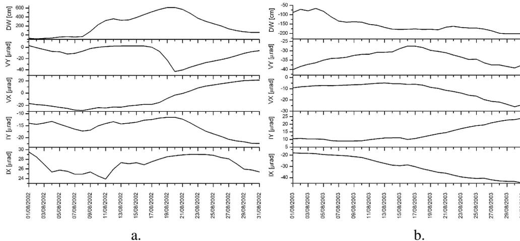
Figure 7 - Connection between the tilt of high bank and the water level variations of the Danube during a strong flood between 10.08.2002 and 25.08.2002 (a) and during a low water level between 07.08.2003 and 31.08.2003 (b). DW = water level of the Danube; VX, VY = tilt components measured at the foot of the high bank; IX, IY = tilt components measured on the top of the high bank
