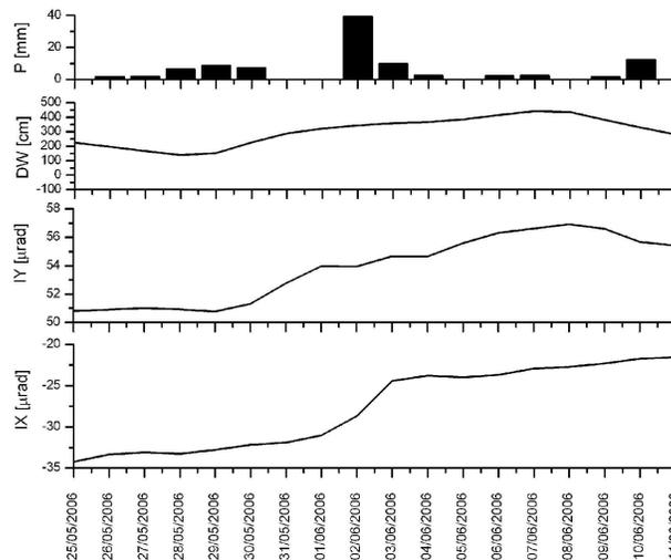
Figure 8 - Example for the influence of the precipitation. P = precipitation; DW = water level of the Danube; IX, IY = tilt components measured on the top of the high bank
