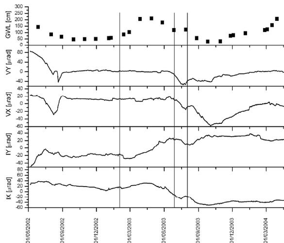
Figure 6 - The influence of the ground water onto the movements of the steep high bank.
