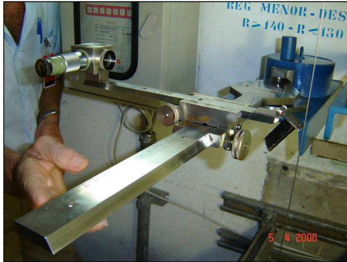
Figure 3 - Plumb line reading at ITAIPU dam with optical coordinometer
