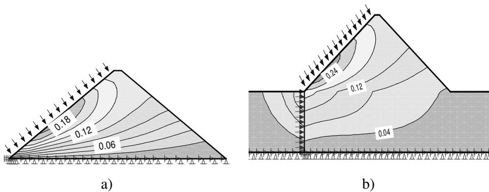
Figure 6: Calculated horizontal displacements (in metres) at the end of the filling of the reservoir for a CFRD of 75 m of height resting on: a) rock; b) 60 m of till (moraine).
