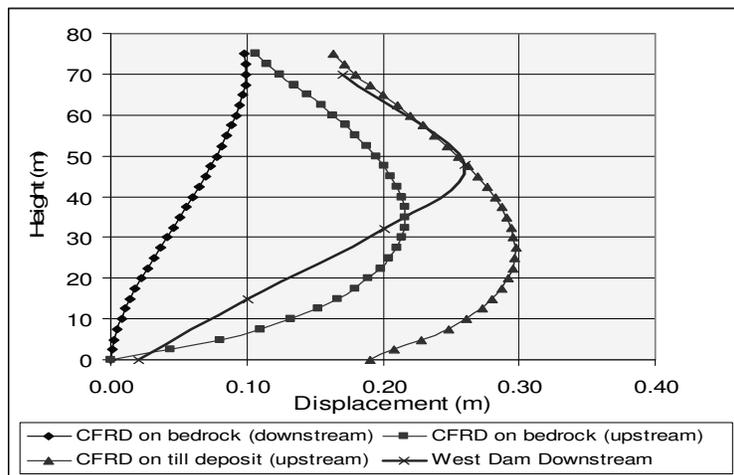
Figure 5: Displacements of CFRD and West Dam at the end of filling up a reservoir
