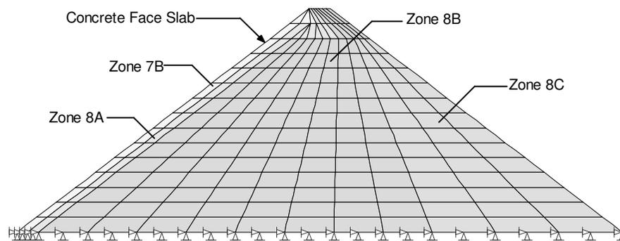
Figure 2: CFRD of 75 m of height resting on bed rock
