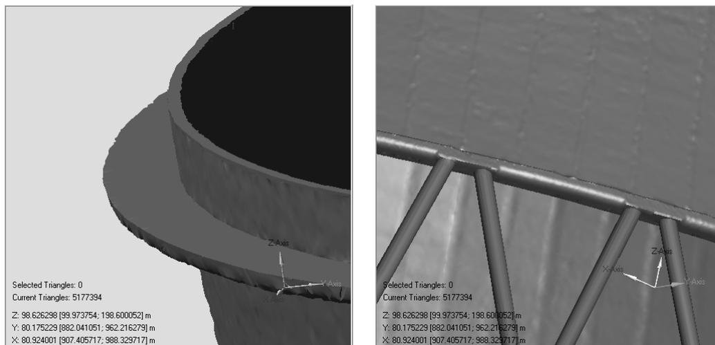
Figure 4: Details of the model of the tower: the cornice (left) and part of the lintel and the diagonals (right)
