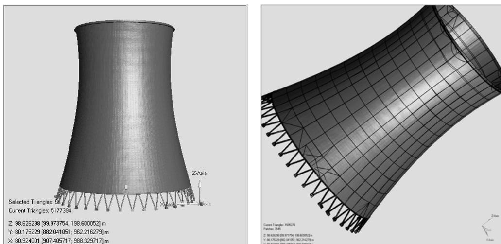
Figure 5: Final polygonal model (left). Patches created for the creation of the NURBS model
