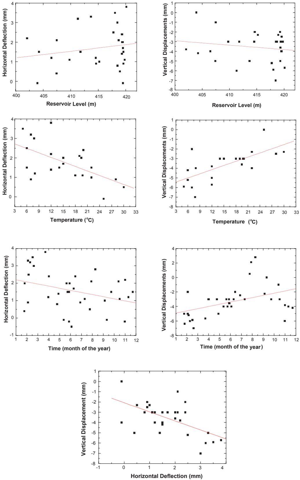
Fig. 3 Diagrams of Horizontal Deflection and Vertical Displacement of Monitoring Station C3 vs Reservoir Level, Temperature and Time. There is no significant linear correlation between these parameters which means that the Ladhon Dam, inspite of its age (> 40 years) is perfectly rigid.
