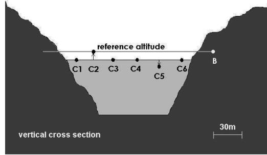
Fig. 2 Relative elevations of each control station is measured relative to reference station B using high accuracy spirit leveling. Vertical displacement in epoch  $i$  is defined on the difference between the elevation of a certain point in period  $j$  and an initial value at epoch 0.
