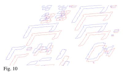
Naturally the question how to determine the height of a building arises here. For the purposes of the three-dimensional model of the populated area, we consider that it is sufficient to set up a medium height of the floor and in this manner to obtain the heights of the buildings. Our system allows us to change the heights of the floors for specific buildings.
