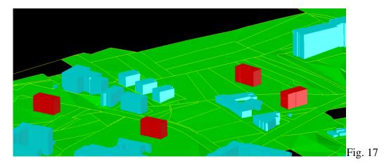
The design positions of new buildings are indicated in red color. As it may be supposed with this technology for creation of three-dimensional models of the populated areas that the distances between the existing buildings are fully precise, within the limits of the precision of the cadastre map, the obtained urbanization design will completely correspond to the existing situation and all the needed data may be obtained from this model.
