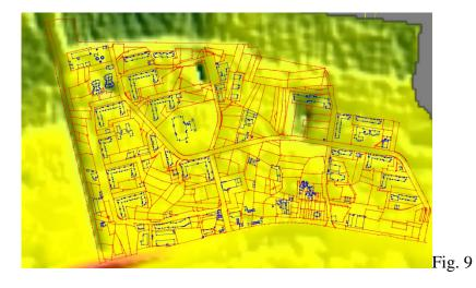
A specialized format is created in Bulgaria - \*.CAD for exchange of data from a digital cadastre map. We will not consider this format in detail, we will only note down that it preserves information about limits of properties, contours of buildings, as well as a number of floors, structure of the buildings and so on. The files in format CAD are text ones, which allows the very easy extraction of information needed with developed applied software.
