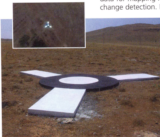
Premark for WorldView-2. Inset shows view of premark from satellite. (Mutluoglu)
